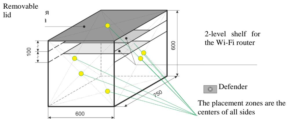
Fig. 1. The diagram of the Faraday cage used in the research showing the location of resonators.
