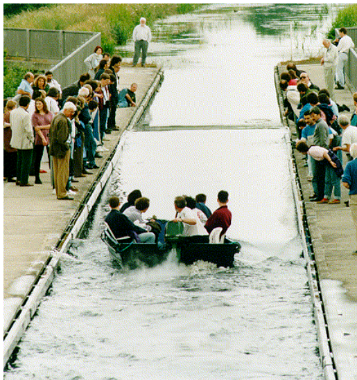
Fig. 3. A soliton wave moving along the channel
