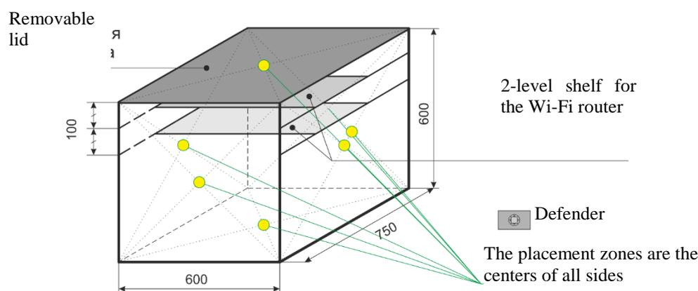
Fig. 1. The diagram of the Faraday cage used in the research showing the location of resonators.
