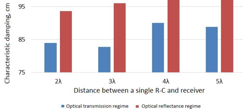
**Fig. 11** The dependence of the characteristic damping versus distance (in  $\lambda$ ) between the R-C and the signals receiver.
