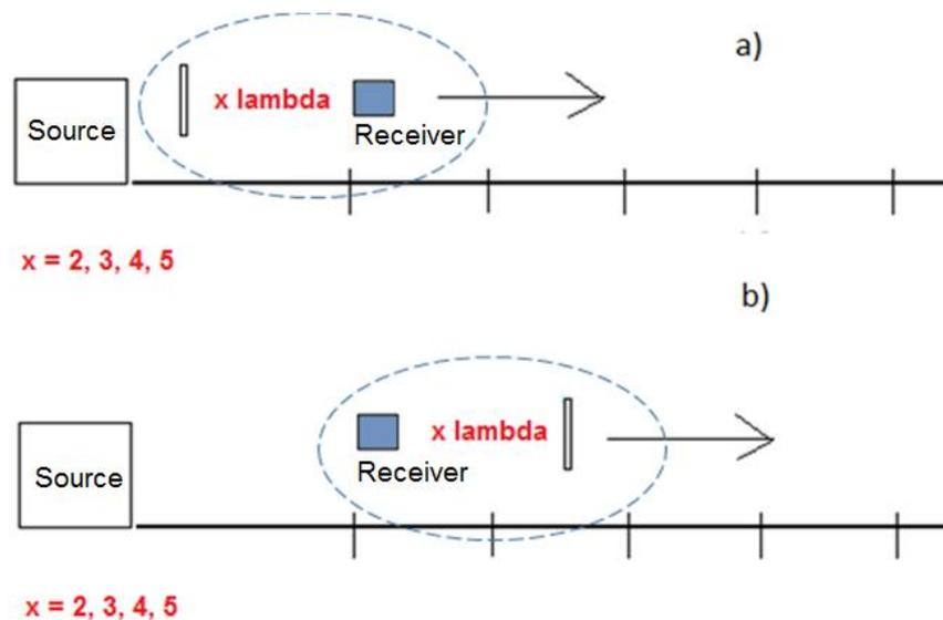
**Fig. 2** Experimental schemes for the testing of radiation power of the radiation source. The resonator-converters positioned at the distance of  $2\lambda - 10\lambda$  in the regimes of: a) optical transmission and b) optical reflection.
