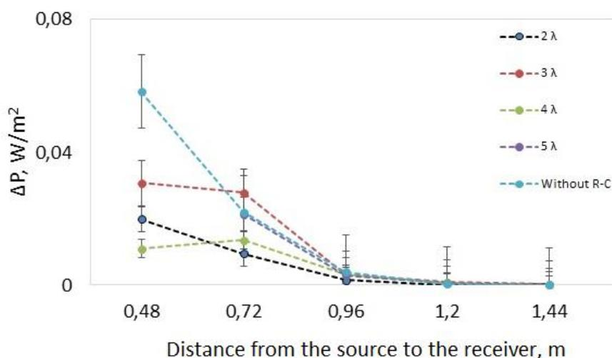
**Fig. 6** The irradiance versus distance of the receiver to the radiation source (800 W, 2.5 GHz). The resonator-converter kept at a distance of 2 - 5  $\lambda$  from the receiver and used in the regime of the optical reflectance.
