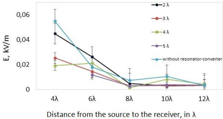
**Fig. 9** The electric field strength measured by the receiver versus the distance to the radiation source, where the group of resonators-converters is in the regime of optical transmission at distance ranging between  $2\lambda$  and  $5\lambda$  from the receiver.
