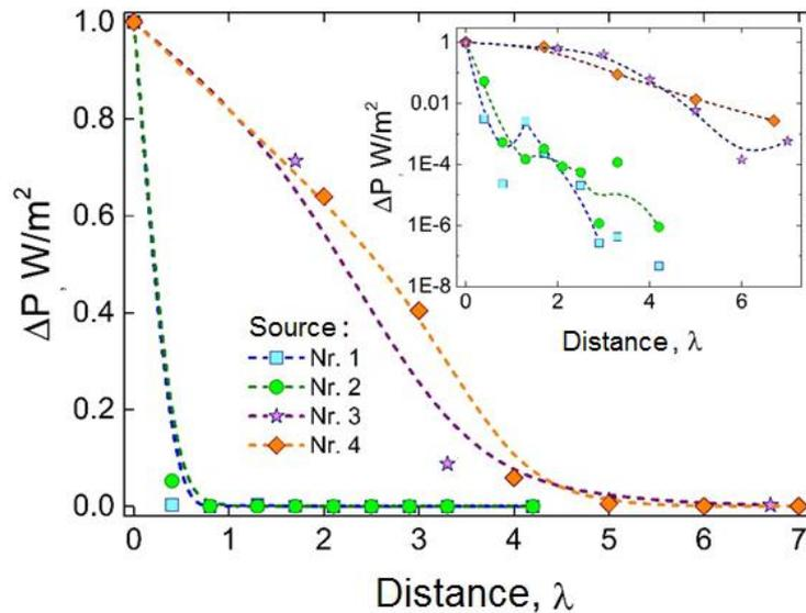
**Fig. 4** The irradiance versus distance between source and receiver dependences in the case of 4 different radiation sources. The resonator-converter positioned at a fixed distance from receiver. Inset represents the semi-log plots of the same dependencies.
