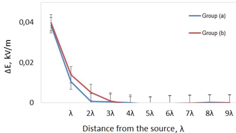
**Fig. 7** The electric field strength versus the distance from the 800 W, 2.5 GHz radiation source dependences measured for two groups of R-Cs. The R-C groups operated in regime of the optical transmission.
