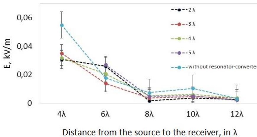
**Fig. 10** The electric field strength measured by the receiver versus the distance to the radiation source, where the group of resonator-converters in the regime of optical reflection at a distance of  $2\lambda - 5\lambda$  from the receiver.
