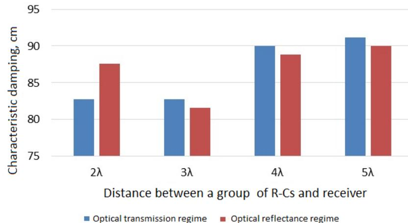
**Fig. 12** The dependence of the characteristic damping of signals versus distance (in  $\lambda$ ) between the group (a) of the R-Cs and the signals receiver.
