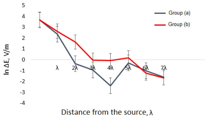
**Fig. 8** A semi-log plot of the same as in Fig. 7 electric field strength versus distance to the radiation source (800 W, 2.5 GHz) dependences. The R-C groups operated in regime of the optical transmission.
