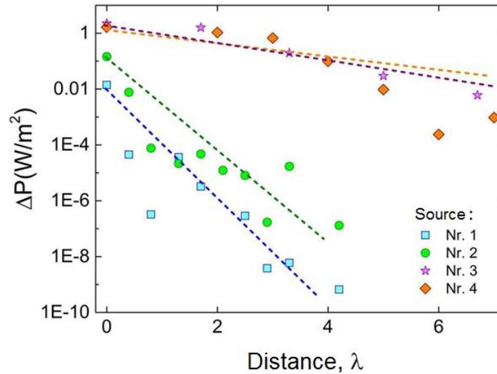
**Fig. 3** A semi-log plot of the relative irradiance of 4 radiation sources versus the distance from a source to the receiver with the resonator-converter, positioned at a fixed distance from the receiver. Dotted lines represent semi-log plot of calculations of  $\Delta P = P_0 - P_{R-C}$  versus distance for each case of the radiation source.
