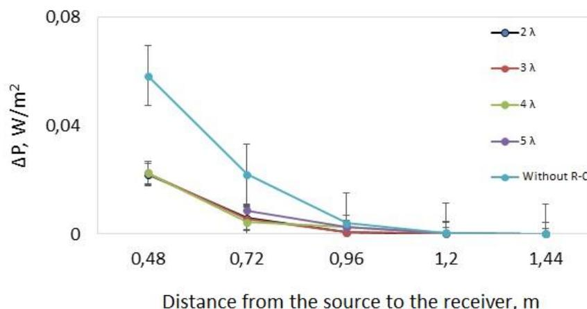
**Fig. 5** The irradiance produced by the radiation source versus distance of receiver from this source dependence measured for the case of 800 W power radiation source emitting frequency band with central frequency of 2.5 GHz. The resonator-converter is in the optical transmission mode positioned at a distance of 2 - 5  $\lambda$  from the receiver.
