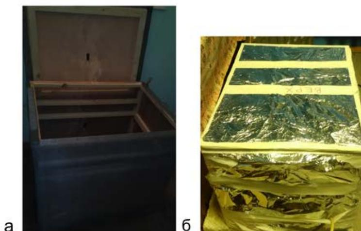
*Fig. 1. A Faraday cage covered in (a) a metal mesh, (b) a metal mesh and aluminum foil.*
