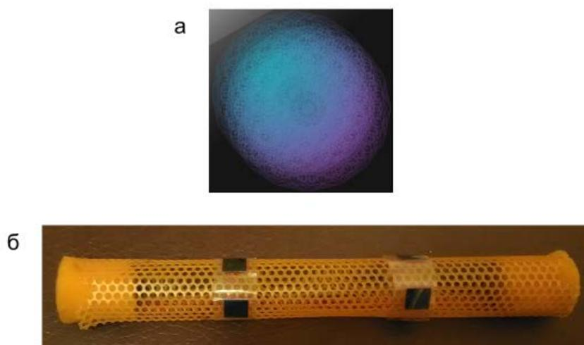
*Fig. 3. A LIFETUNE microprocessor (a) and an experimental mesh test tube for bees with microprocessors located on it (b).*
